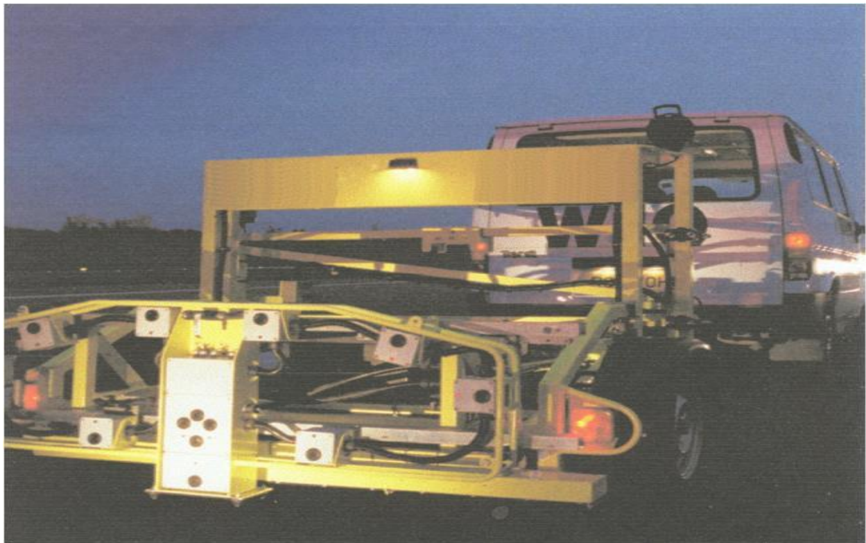
Figure 17-4. An example of mobile measuring equipment
